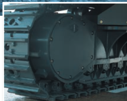
Sturdy travel motor guards and rock protectors
