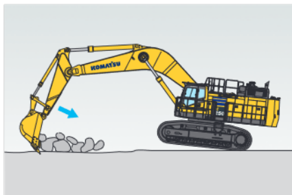
Power mode Boom pushing force is increased, providing a higher penetration force.
