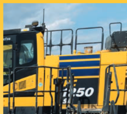
Hand rails and anti-slip plates
