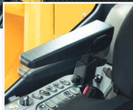
Armrest with simple height adjustment
